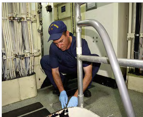
LCDR Matt Dooris conducting lead sampling to confirm if any lead dust from bilge area is being tracked into other areas of the ship. Photo by Auxiliarist Eric Eltinge, HSWL SC (se-fo) Detached San Pedro
