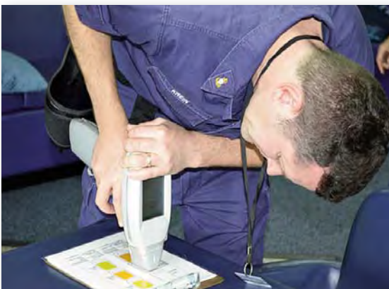
Before going onboard, all testing equipment must be calibrated. Here, MSTC Tristan Krein confirms all readings of the NITON Portable X-Ray Fluorescence (XRF) Analyzer "lead gun" are within manufacturer's specifications. Photo by Auxiliarist Eric Eltinge, HSWL SC (se-fo) Detached San Pedro.
